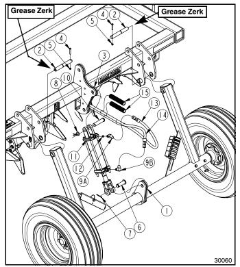
Rear Axle & Lift Cylinder Assembly Figure 1-3
